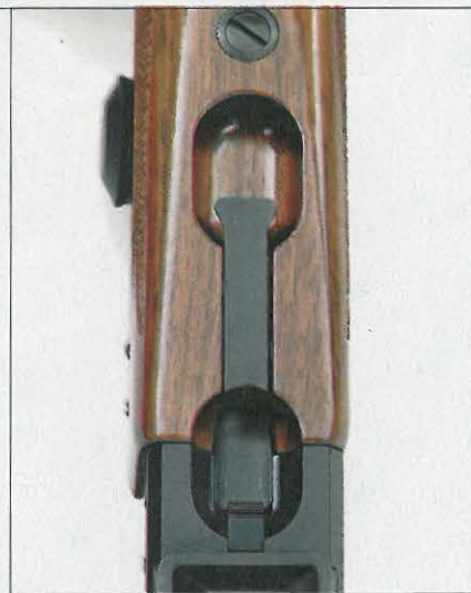
The takedown lever allows instant disassembly, a real plus for situations where storage space is limited.
